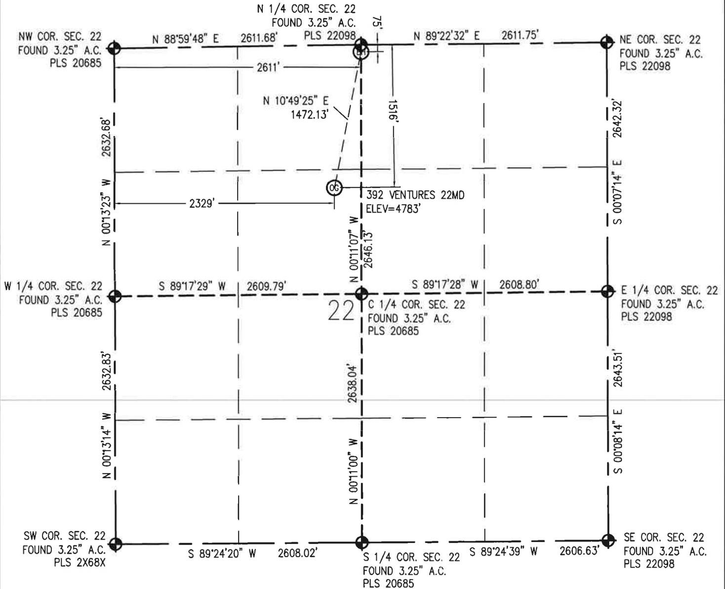
IN ACCORDANCE WITH A REQUEST FROM RICH BARTELS - RBF MINERALS, BASELINE ENGINEERING CORP. HAS DETERMINED THE LOCATION OF THE 392 VENTURES 22MD TO BE 1,516' FNL AND 2,329' FWL, AS MEASURED AT NINETY (90) DEGREES FROM THE SECTION LINE OF SECTION 22, TOWNSHIP 6 NORTH, RANGE 67 WEST AND THE BOTTOM HOLE LOCATION TO BE 75' FNL AND 2,611' FWL OF SECTION 22, TOWNSHIP 6 NORTH, RANGE 67 WEST, 6TH PRINCIPAL MERIDIAN, WELD COUNTY, COLORADO.
