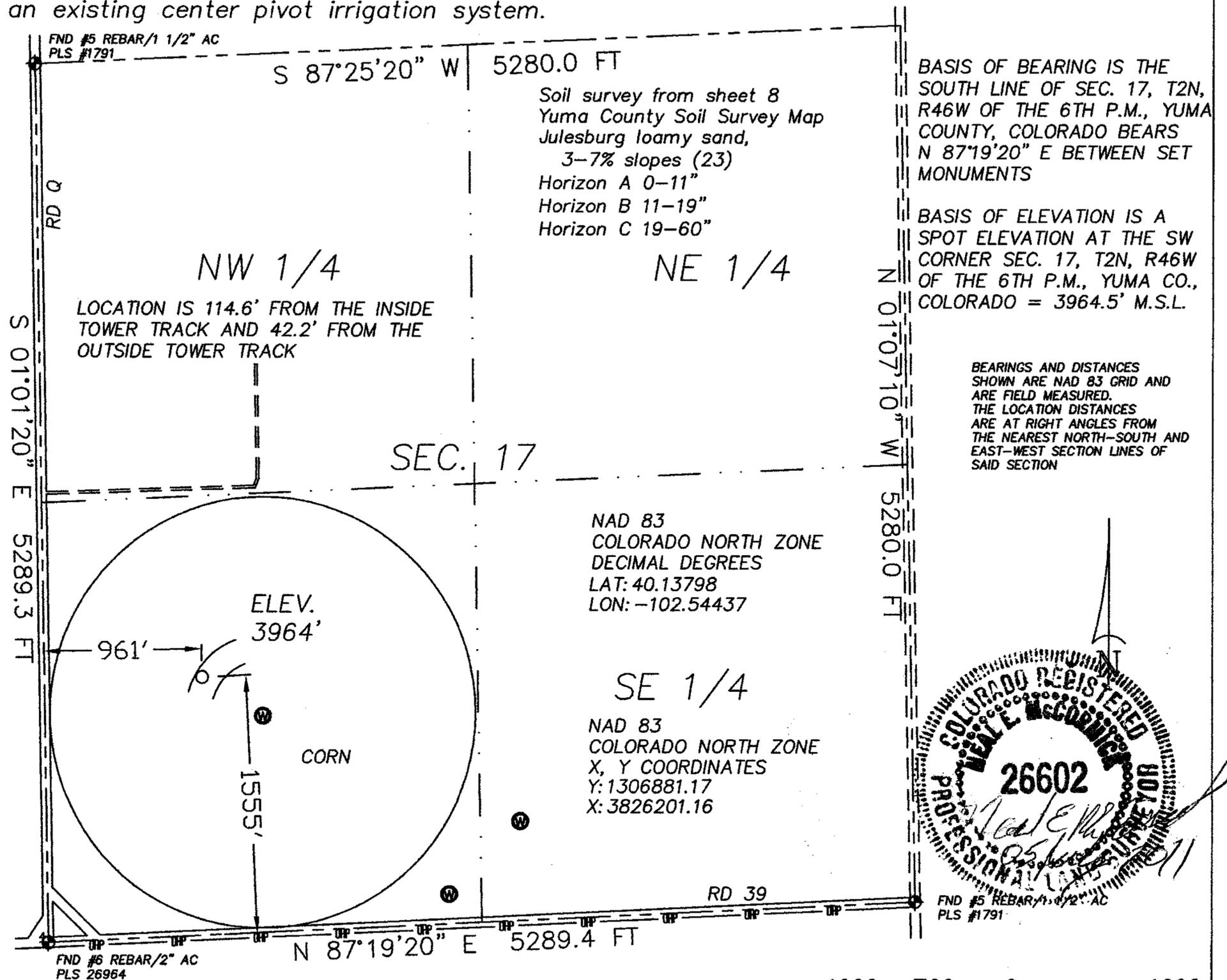
BEARINGS AND DISTANCES SHOWN ARE NAD 83 GRID AND ARE FIELD MEASURED. THE LOCATION DISTANCES ARE AT RIGHT ANGLES FROM THE NEAREST NORTH-SOUTH AND EAST-WEST SECTION LINES OF SAID SECTION
