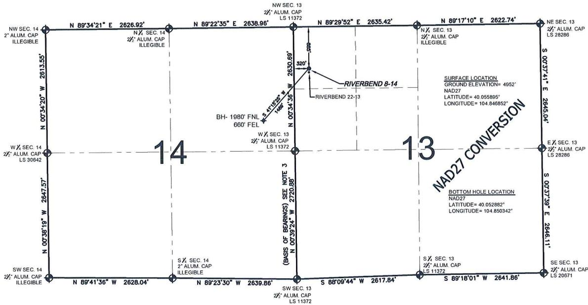
WELL RIVERBEND 8-14 TO BE LOCATED 885' FNL AND 320' FWL, SECTION 13, T1N, R67W OF THE 6th P.M.
