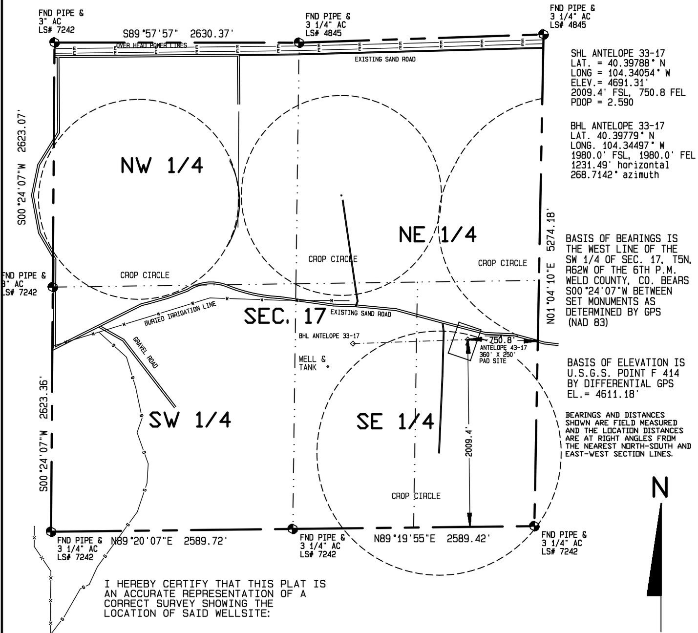
I HEREBY CERTIFY THAT THIS PLAT IS AN ACCURATE REPRESENTATION OF A CORRECT SURVEY SHOWING THE LOCATION OF SAID WELLSITE:
