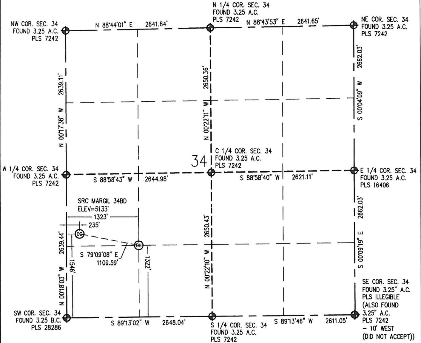
IN ACCORDANCE WITH A REQUEST FROM CRAIG RASMUSON - SYNERGY RESOURCES, BASELINE ENGINEERING CORP. HAS DETERMINED THE LOCATION OF THE SRC MARGIL 34BD TO BE 1,546' FSL AND 235' FWL, AS MEASURED AT NINETY (90) DEGREES FROM THE SECTION LINE OF SECTION 34, TOWNSHIP 4 NORTH, RANGE 68 WEST AND THE BOTTOM HOLE LOCATION TO BE 1,322' FSL AND 1,323' FWL OF SECTION 34, TOWNSHIP 4 NORTH, RANGE 68 WEST, 6TH PRINCIPAL MERIDIAN, WELD COUNTY, COLORADO.
