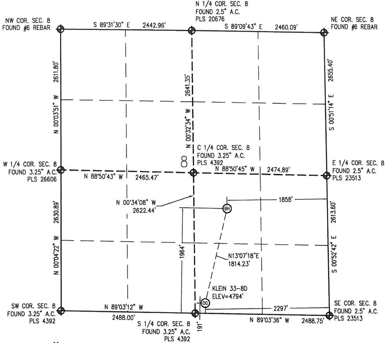
IN ACCORDANCE WITH A REQUEST FROM CRAIG RASMUSON - SYNERGY RESOURCES, BASELINE ENGINEERING CORP. HAS DETERMINED THE LOCATION OF THE KLEIN 33-8D TO BE 191' FSL AND 2,297' FEL, AS MEASURED AT NINETY (90) DEGREES FROM THE SECTION LINE OF SECTION 8, TOWNSHIP 4 NORTH, RANGE 67 WEST AND THE BOTTOM HOLE LOCATION TO BE 1,964' FSL AND 1,858' FEL OF SECTION 8, TOWNSHIP 4 NORTH, RANGE 67 WEST, 6TH PRINCIPAL MERIDIAN, WELD COUNTY, COLORADO.
