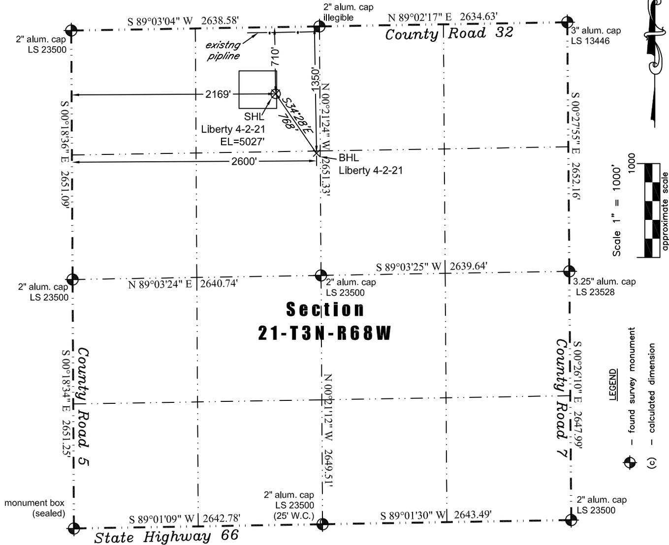
In accordance with a request from Dave Bale of EnCana Oil & Gas (USA) Inc., PLS Group, LLC has determined the location of the **Liberty 4-2-21** well site to be SHL 710' FNL and 2169' FWL (BHL 1350' FNL and 2600' FWL) as measured at ninety (90) degrees from the section lines of Section 21, Township 3 North, Range 68 West of the 6th Principal Meridian, Weld County, Colorado.
