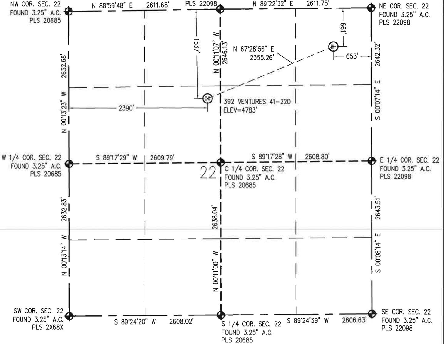
IN ACCORDANCE WITH A REQUEST FROM RICH BARTELS - RBF MINERALS, BASELINE ENGINEERING CORP. HAS DETERMINED THE LOCATION OF THE 392 VENTURES 41-22D TO BE 1,537' FNL AND 2,390' FWL, AS MEASURED AT NINETY (90) DEGREES FROM THE SECTION LINE OF SECTION 22, TOWNSHIP 6 NORTH, RANGE 67 WEST AND THE BOTTOM HOLE LOCATION TO BE 661' FNL AND 653' FEL OF SECTION 22, TOWNSHIP 6 NORTH, RANGE 67 WEST, 6TH PRINCIPAL MERIDIAN, WELD COUNTY, COLORADO.
