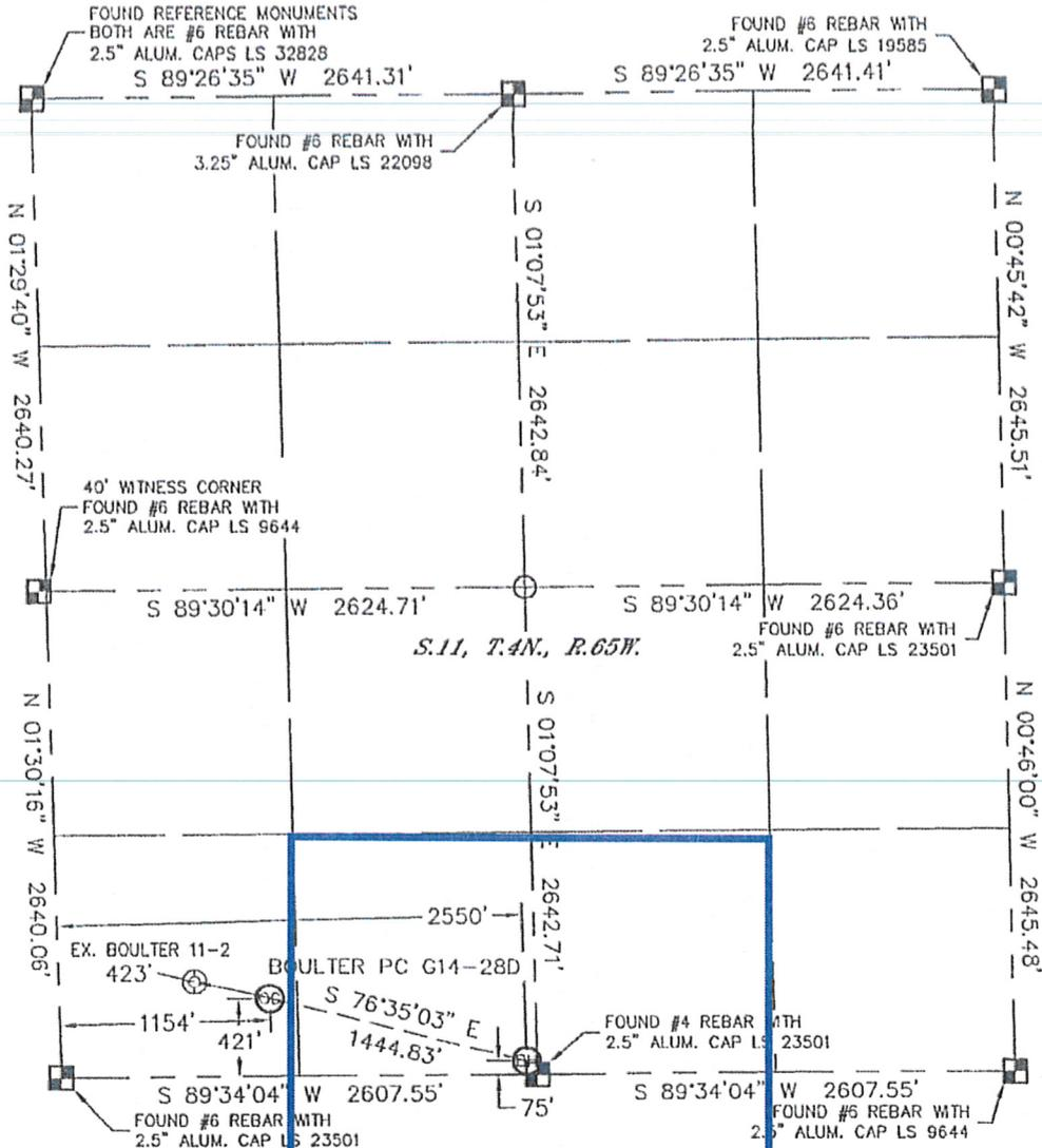
In accordance with a request from Ryan Antonio with Noble Energy Inc., Lat40°, LLC has determined the surface location of the BOULTER PC G14-28D to be 421' from the SOUTH line and 1154' from the WEST line and the bottom hole to be 75' from the SOUTH line and 2550' from the WEST line as measured at right angles from the section lines of Section 11, Township 4 North, Range 65 West of the Sixth Principal Meridian, County of Weld, State of Colorado.
