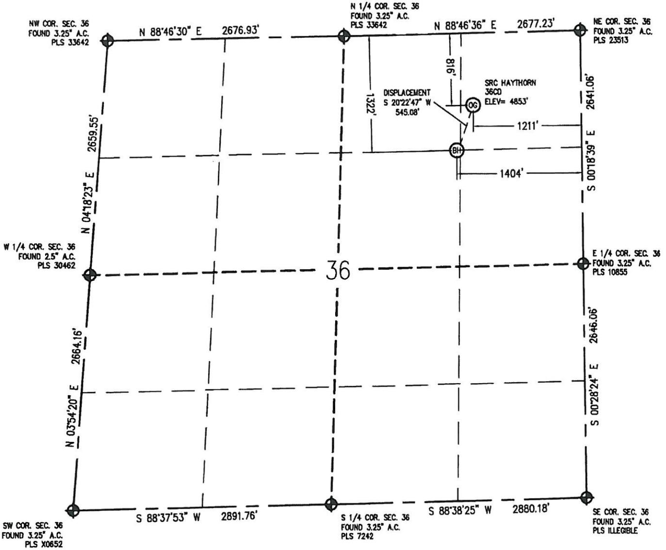
IN ACCORDANCE WITH A REQUEST FROM CRAIG RASMUSON - SYNERGY RESOURCES CORP., BASELINE ENGINEERING CORP. HAS DETERMINED THE LOCATION OF THE SRC HAYTHORN 36CD TO BE 816' FNL AND 1211' FEL, AS MEASURED AT NINETY (90) DEGREES FROM THE SECTION LINE OF SECTION 36, TOWNSHIP 7 NORTH, RANGE 66 WEST AND THE BOTTOM HOLE LOCATION TO BE 1322' FNL AND 1404' FEL OF SECTION 36, TOWNSHIP 7 NORTH, RANGE 66 WEST, 6TH PRINCIPAL MERIDIAN, WELD COUNTY, COLORADO.
