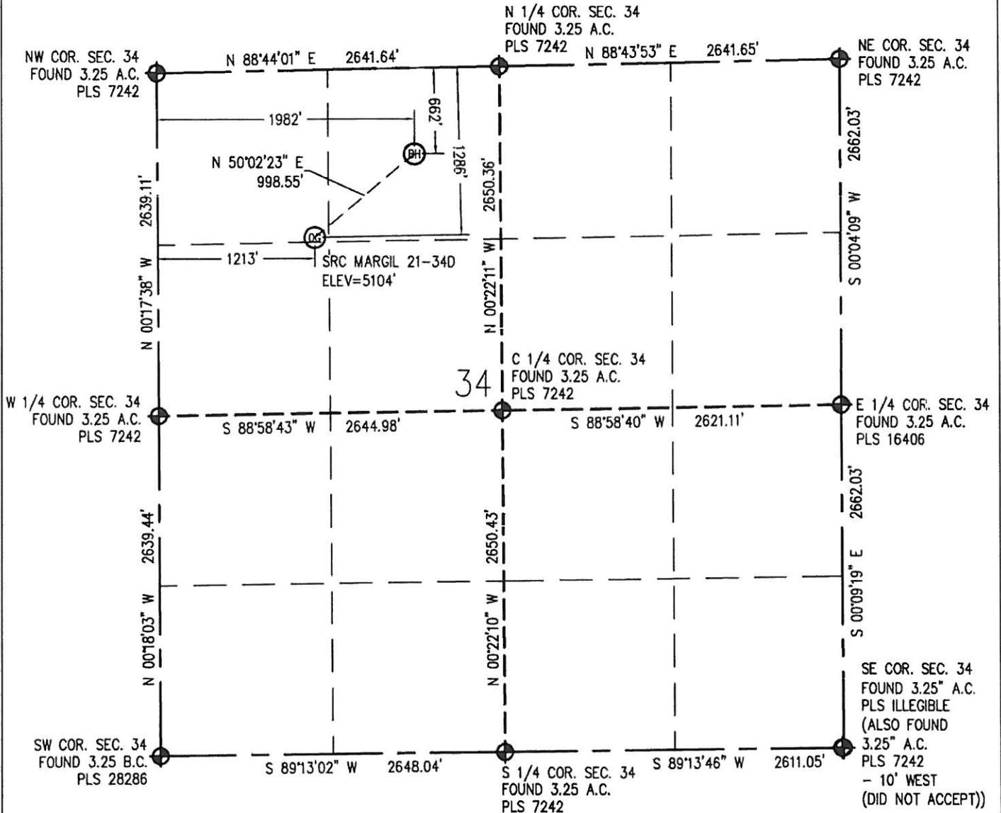
IN ACCORDANCE WITH A REQUEST FROM CRAIG RASMUSON - SYNERGY RESOURCES, BASELINE ENGINEERING CORP. HAS DETERMINED THE LOCATION OF THE SRC MARGIL 21-34D TO BE 1,286' FNL AND 1,213' FWL, AS MEASURED AT NINETY (90) DEGREES FROM THE SECTION LINE OF SECTION 34, TOWNSHIP 4 NORTH, RANGE 68 WEST AND THE BOTTOM HOLE LOCATION TO BE 662' FNL AND 1,982' FWL OF SECTION 34, TOWNSHIP 4 NORTH, RANGE 68 WEST, 6TH PRINCIPAL MERIDIAN, WELD COUNTY, COLORADO.
