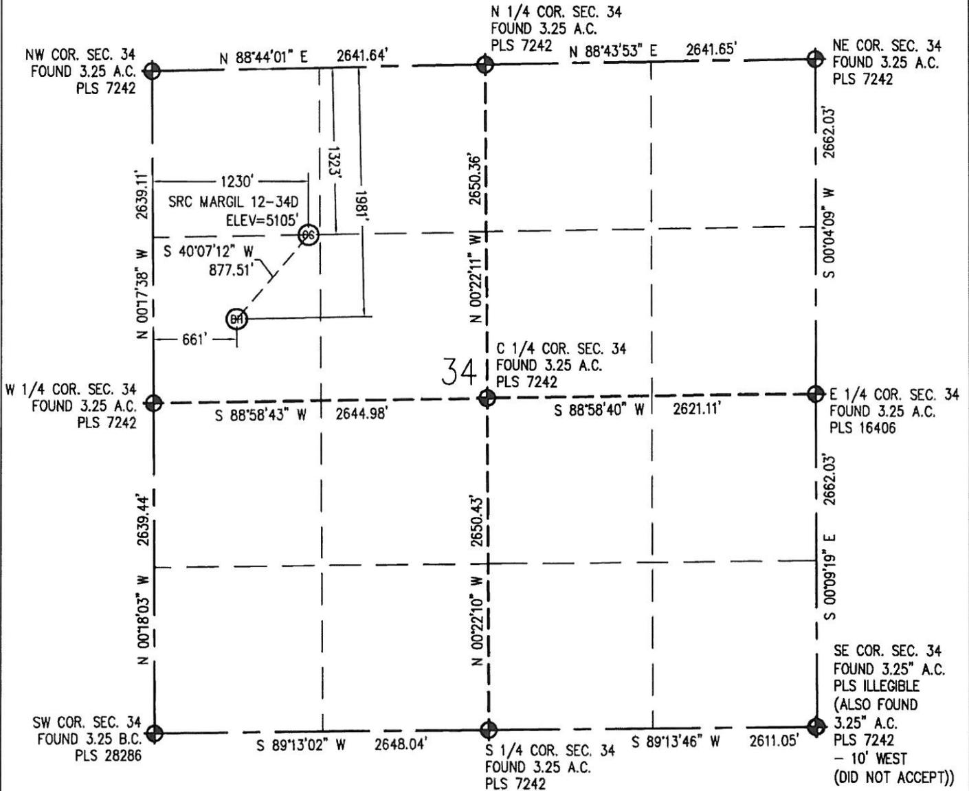
IN ACCORDANCE WITH A REQUEST FROM CRAIG RASMUSON - SYNERGY RESOURCES, BASELINE ENGINEERING CORP. HAS DETERMINED THE LOCATION OF THE SRC MARGIL 12-34D TO BE 1,323' FNL AND 1,230' FWL, AS MEASURED AT NINETY (90) DEGREES FROM THE SECTION LINE OF SECTION 34, TOWNSHIP 4 NORTH, RANGE 68 WEST AND THE BOTTOM HOLE LOCATION TO BE 1,981' FNL AND 661' FWL OF SECTION 34, TOWNSHIP 4 NORTH, RANGE 68 WEST, 6TH PRINCIPAL MERIDIAN, WELD COUNTY, COLORADO.
