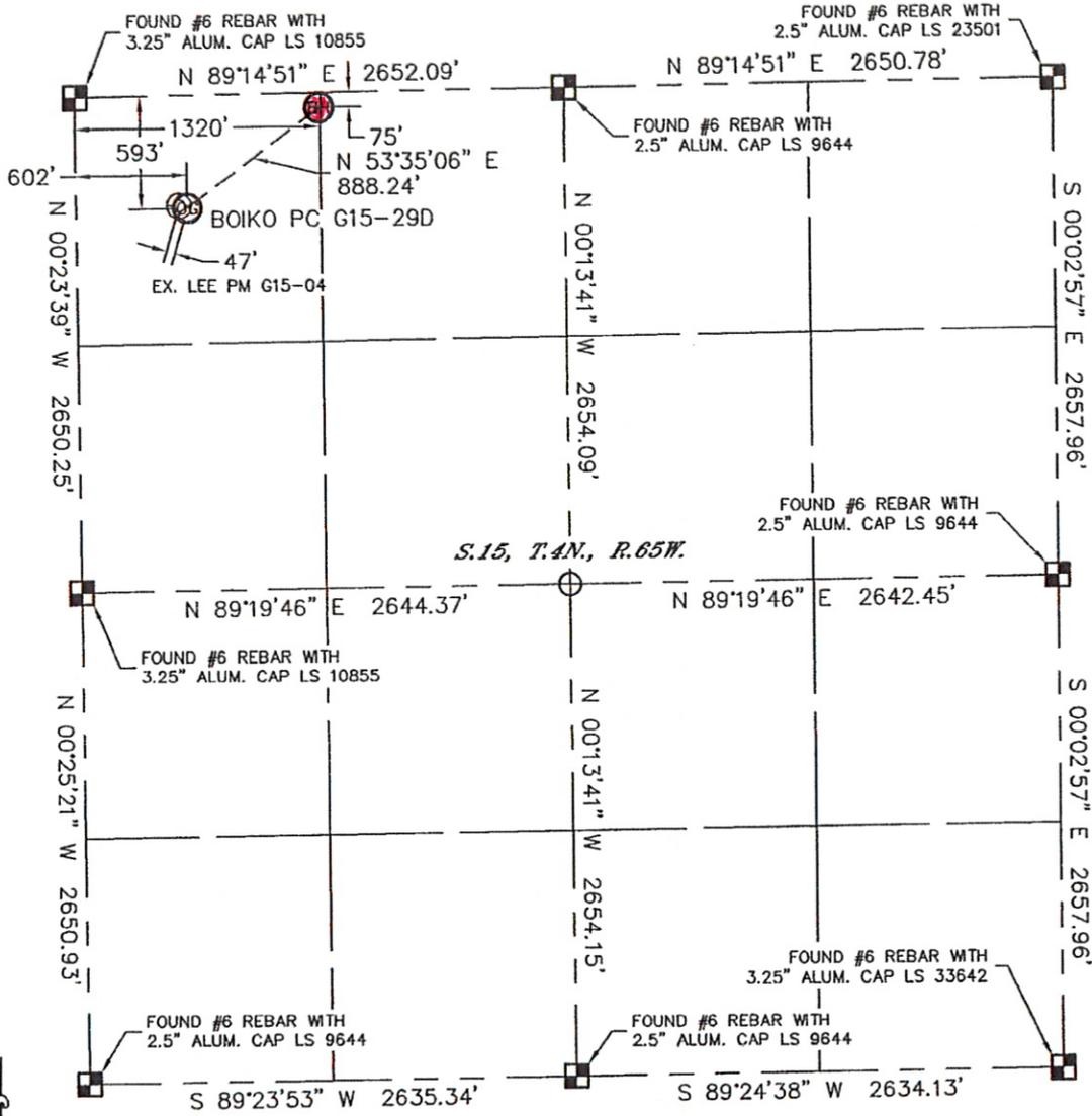
In accordance with a request from Matt Campbell with Noble Energy Inc. Lat40°, Inc. has determined the surface location of the BOIKO\_PC\_G15-29D to be 593' from the NORTH line and 602' from the WEST line and the bottom hole to be 75' from the NORTH line and 1320' from the WEST line as measured at right angles from the section lines of Section 15, Township 4 North, Range 65 West of the Sixth Principal Meridian, County of Weld, State of Colorado.
