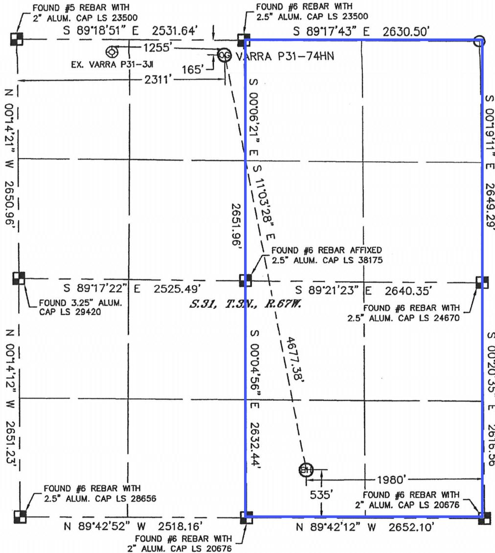
In accordance with a request from Erik Van Decar with Noble Energy Inc., Lat40°, Inc. has determined the surface location of the VARRA P31-74HN to be 165' from the NORTH line and 2311' from the WEST line and the bottom hole to be 535' from the SOUTH line and 1980' from the EAST line as measured at right angles from the section lines of Section 31, Township 3 North, Range 67 West of the Sixth Principal Meridian, County of Weld, State of Colorado.
