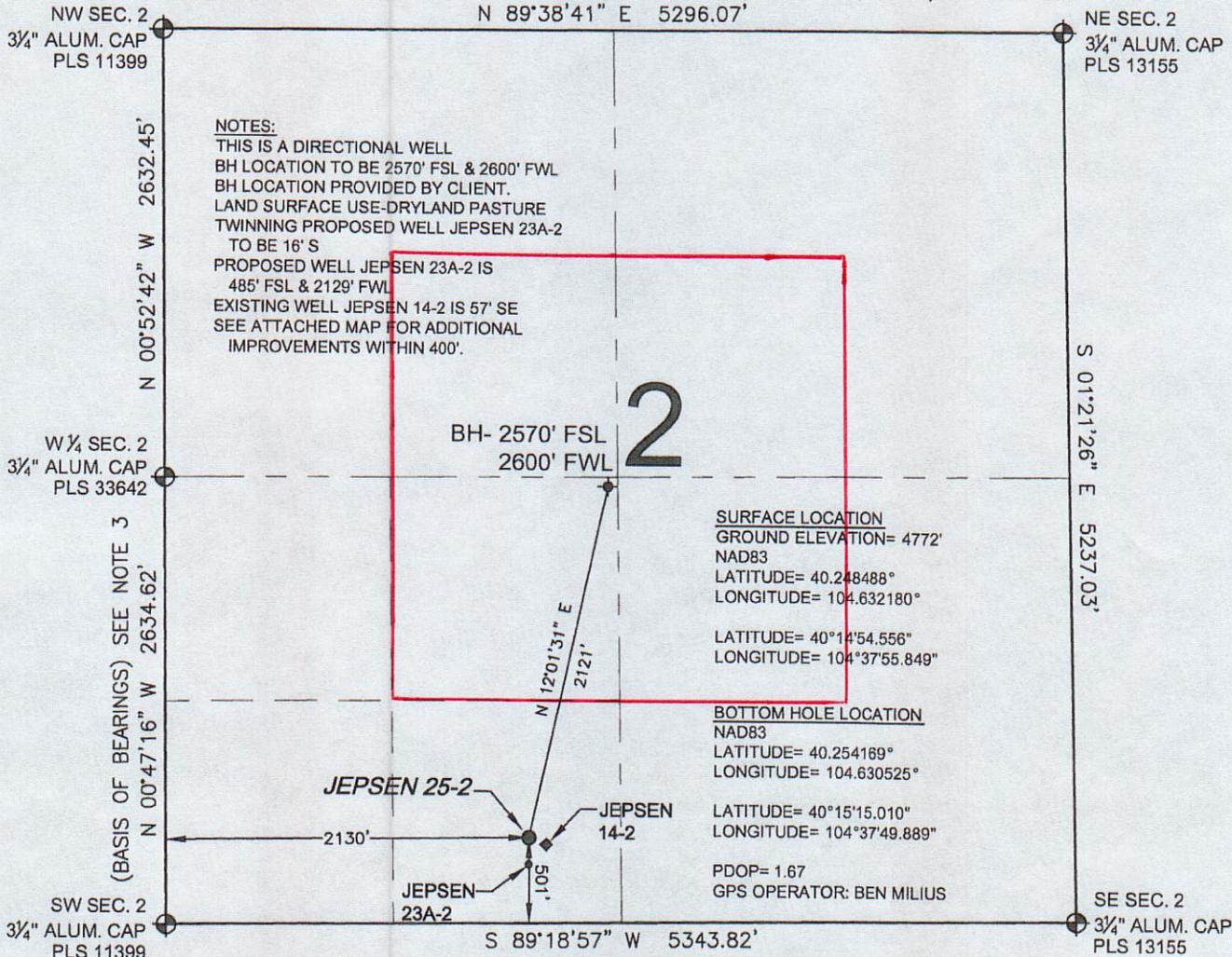
WELL JEPSEN 25-2 TO BE LOCATED 501' FSL AND 2130' FWL, SECTION 2, T3N, R65W OF THE 6th P.M.
