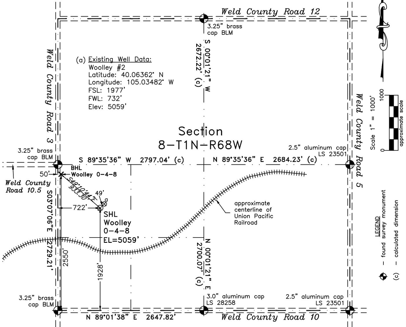
In accordance with a request from Doug Pearlman of EnCana Oil & Gas (USA) Inc., PLS Group, LLC has determined the location of the **Woolley 0-4-8** well site to be SHL: 1928' FSL and 722' FWL, (BHL 2550' FSL and 722' FWL) as measured at ninety (90) degrees from the section lines of Section 8, Township 1 North, Range 68 West, 6th Principal Meridian, County of Weld, CO.
