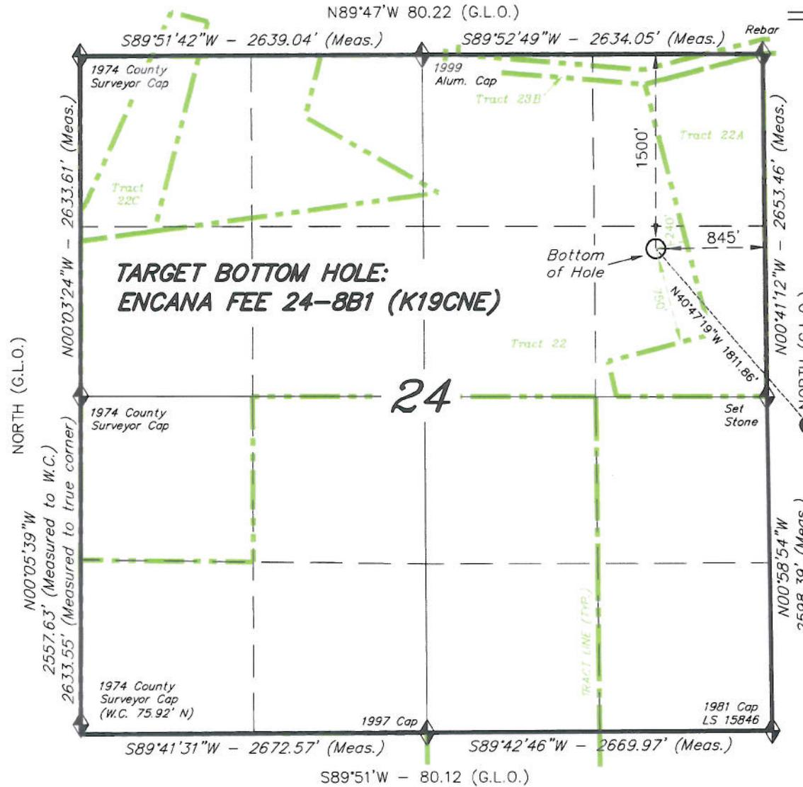
TARGET BOTTOM HOLE, ENCANA FEE 24-8B1 (K19CNE), LOCATED AS SHOWN IN THE SE 1/4 NE 1/4 OF SECTION 24, T6S, R93W, 6th P.M. GARFIELD COUNTY, COLORADO.
