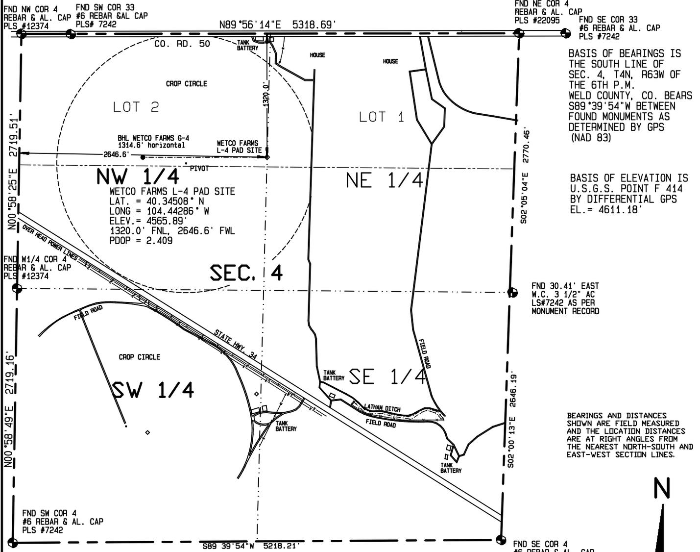
BASIS OF BEARINGS IS THE SOUTH LINE OF SEC. 4, T4N, R63W OF THE 6TH P.M. WELD COUNTY, CO. BEARS S89°39'54"W BETWEEN FOUND MONUMENTS AS DETERMINED BY GPS (NAD 83)
