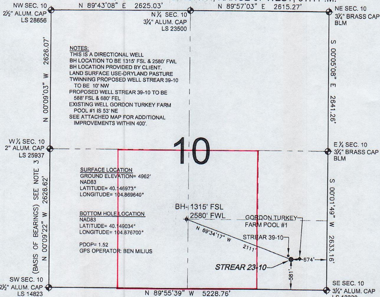
WELL **STREAR 23-10** TO BE LOCATED 581' FSL AND 674' FEL, SECTION 10, T2N, R67W OF THE 6th P.M.
