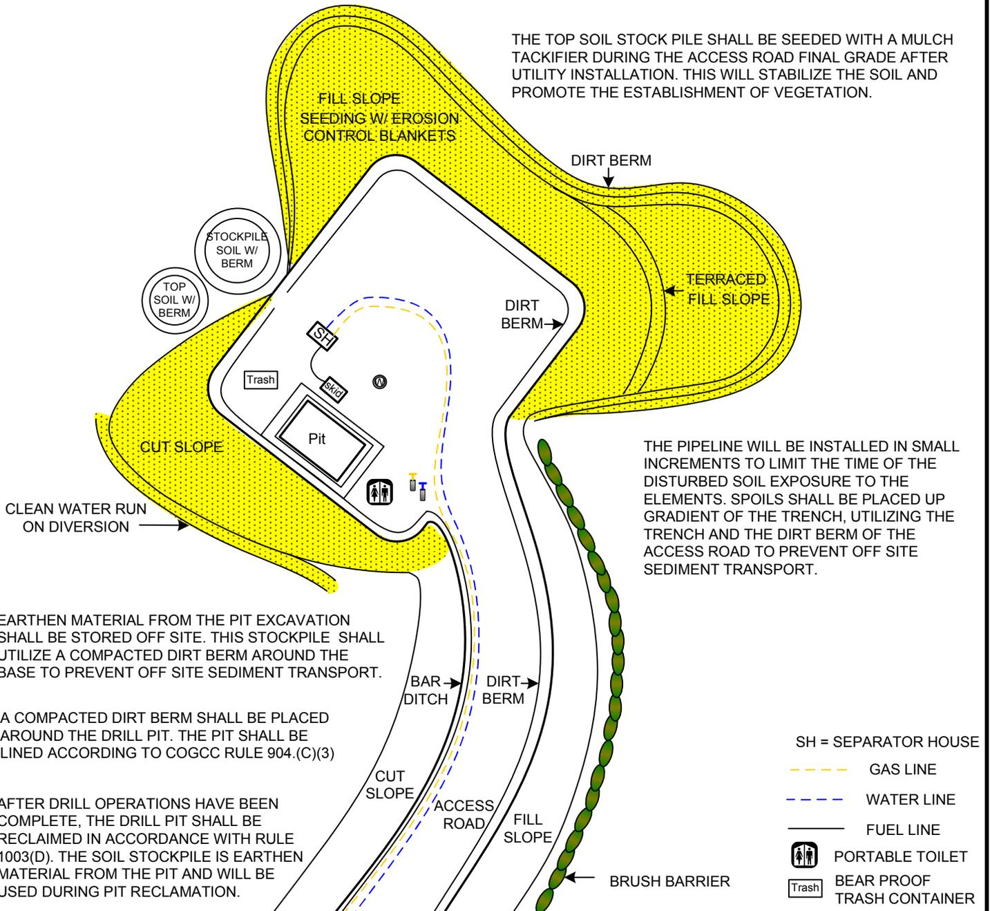
EARTHEN MATERIAL FROM THE PIT EXCAVATION SHALL BE STORED OFF SITE. THIS STOCKPILE SHALL UTILIZE A COMPACTED DIRT BERM AROUND THE BASE TO PREVENT OFF SITE SEDIMENT TRANSPORT.
