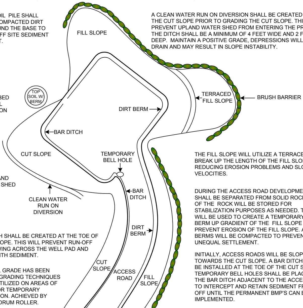
A BAR DITCH SHALL BE CREATED AT THE TOE OF THE CUT SLOPE. THIS WILL PREVENT RUN-OFF FROM FLOWING ACROSS THE WELL PAD AND LOADING WITH SEDIMENT.
