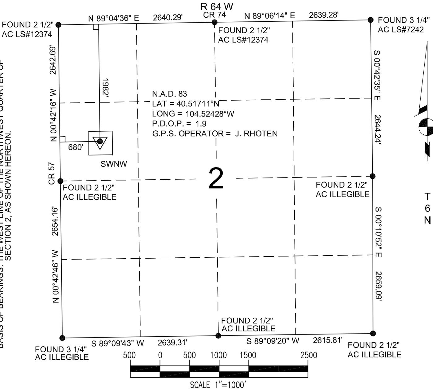
POWER SURVEYING COMPANY, INC. OF FREDERICK, COLORADO HAS IN ACCORDANCE WITH A REQUEST FROM JIM JENSEN OF ST JAMES OIL DETERMINED THE LOCATION OF DYER 2-2 TO BE 1982' FNL & 680' FWL OF SECTION 2, TOWNSHIP 6 NORTH, RANGE 64 WEST OF THE 6th PRINCIPAL MERIDIAN, COUNTY OF WELD, STATE OF COLORADO.
