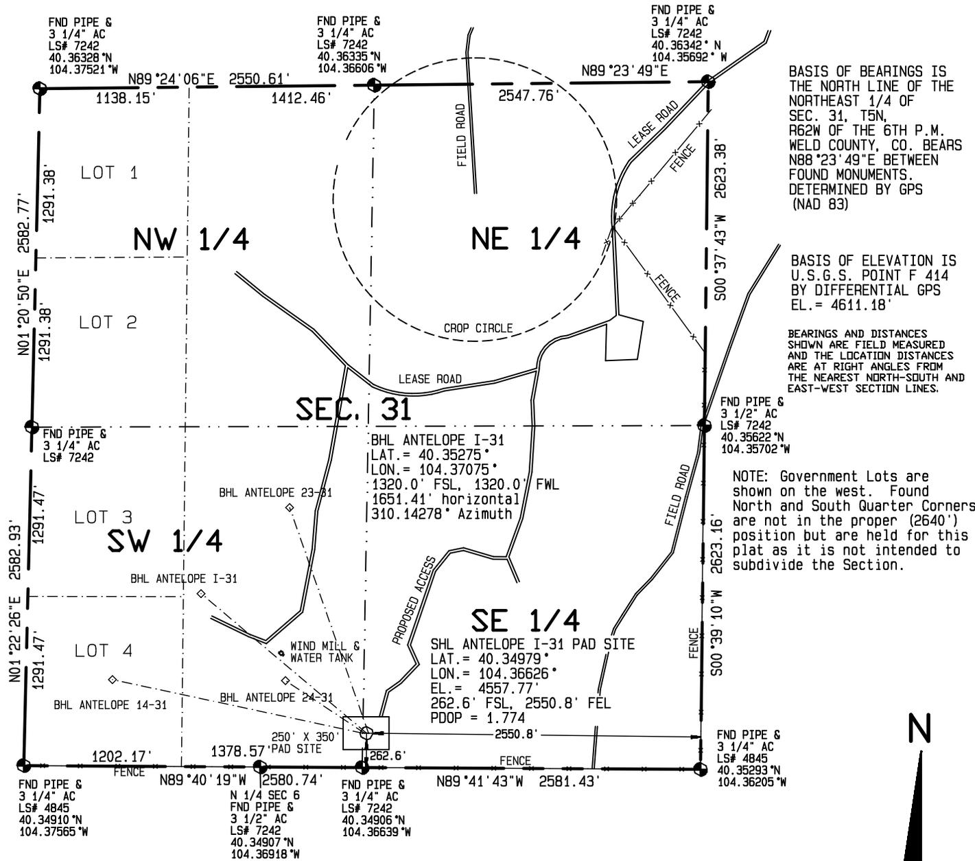
BASIS OF BEARINGS IS THE NORTH LINE OF THE NORTHEAST 1/4 OF SEC. 31, T5N, R62W OF THE 6TH P.M. WELD COUNTY, CO. BEARS N88°23'49"E BETWEEN FOUND MONUMENTS. DETERMINED BY GPS (NAD 83)
