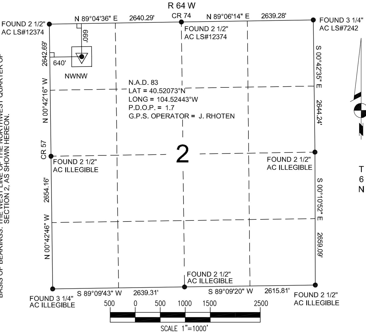
POWER SURVEYING COMPANY, INC. OF FREDERICK, COLORADO HAS IN ACCORDANCE WITH A REQUEST FROM JIM JENSEN OF ST JAMES OIL DETERMINED THE LOCATION OF DYER 1-2 TO BE 660' FNL & 640' FWL OF SECTION 2, TOWNSHIP 6 NORTH, RANGE 64 WEST OF THE 6th PRINCIPAL MERIDIAN, COUNTY OF WELD, STATE OF COLORADO.
