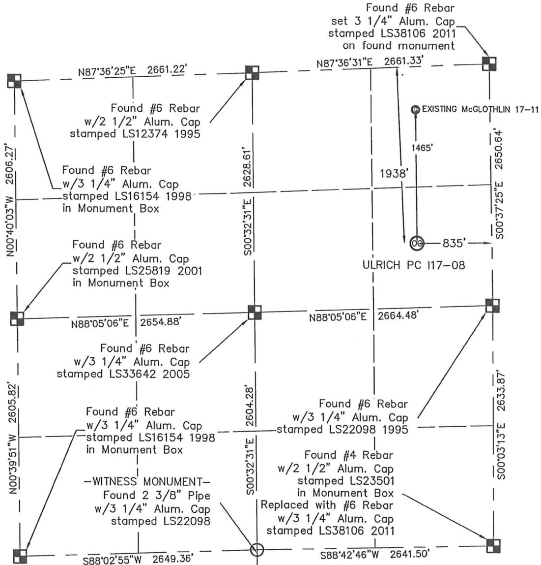
In accordance with a request from RYAN ANTONIO with NOBLE ENERGY INC. King Surveyors Inc. has determined the surface location of the ULRICH PC 117-08 to be 1938' from the NORTH line and 835' from the EAST line, as measured at right angles, from the section lines of Section 17, Township 6 North, Range 66 West of the Sixth Principal Meridian, County of Weld, State of Colorado.
