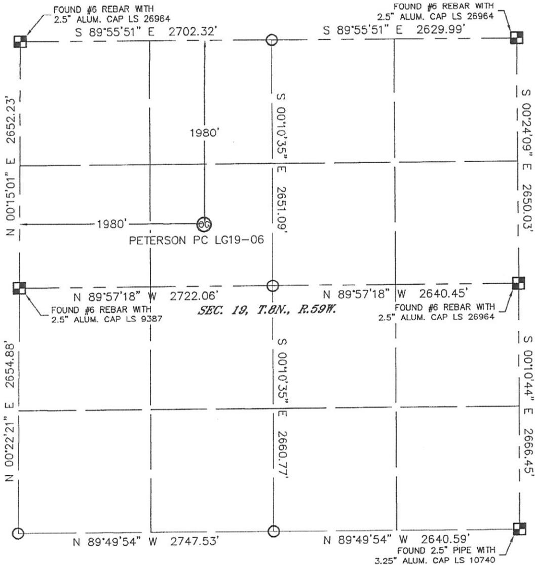
In accordance with a request from Nate McCorkell with Noble Energy Inc., Lat40°, Inc. has determined the surface location of the PETERSON PC LG19-06 to be 1980' from the NORTH line and 1980' from the WEST line as measured at right angles from the section lines of Section 19, Township 8 North, Range 59 West of the Sixth Principal Meridian, County of Weld, State of Colorado.
