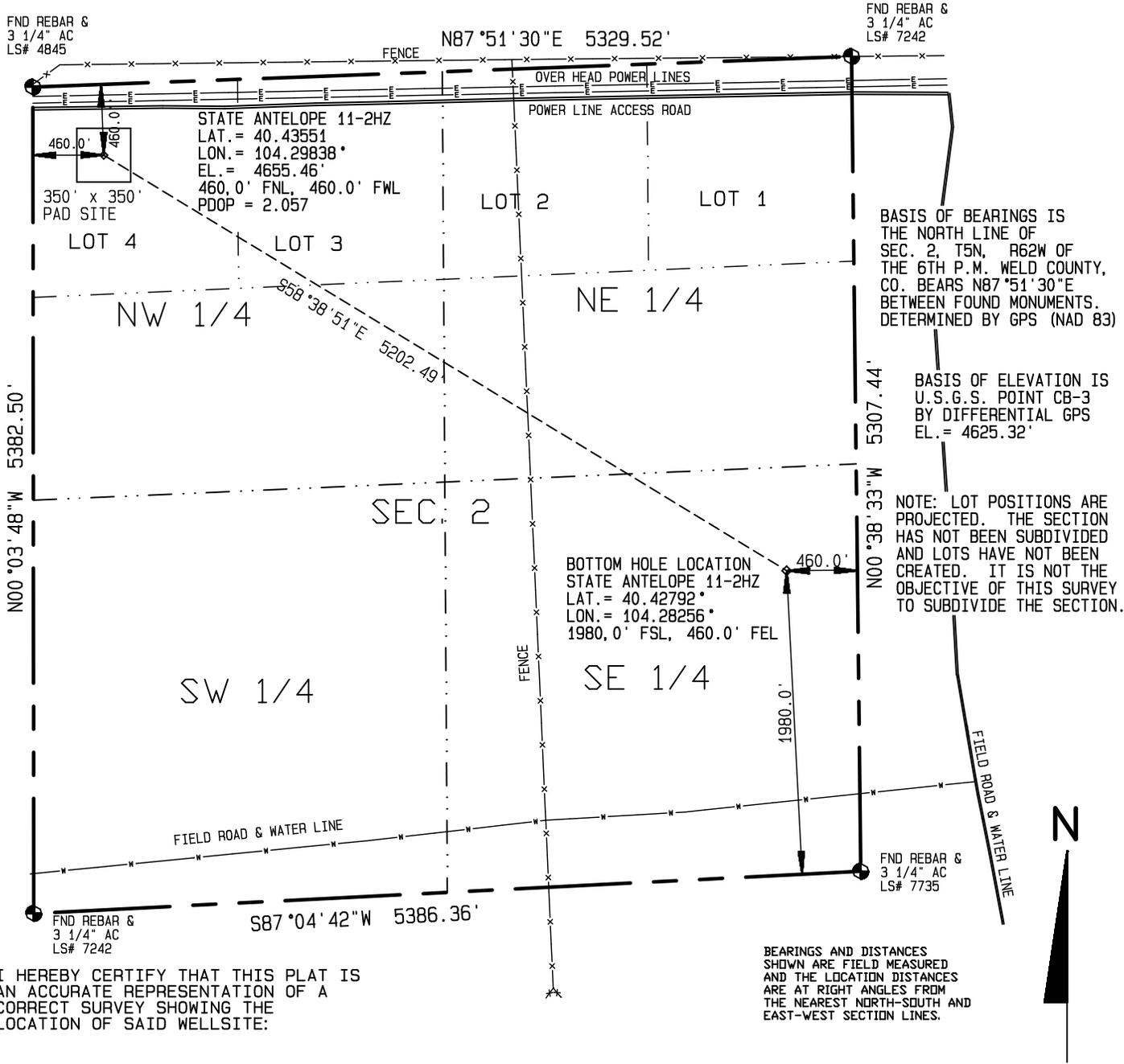
I HEREBY CERTIFY THAT THIS PLAT IS AN ACCURATE REPRESENTATION OF A CORRECT SURVEY SHOWING THE LOCATION OF SAID WELLSITE:
