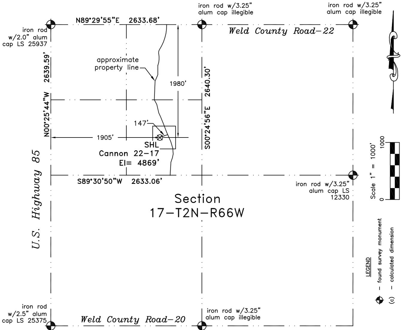
In accordance with a request from Dan Nelson of EnCana Oil & Gas (USA) Inc., PLS Group, LLC has determined the location of the Cannon 22-17 well site to be SHL: 1980' FNL and 1905' FWL, as measured at ninety (90) degrees from the section lines of Section 17, Township 2 North, Range 66 West, 6th Principal Meridian, Town of Erie, County of Weld, CO.
