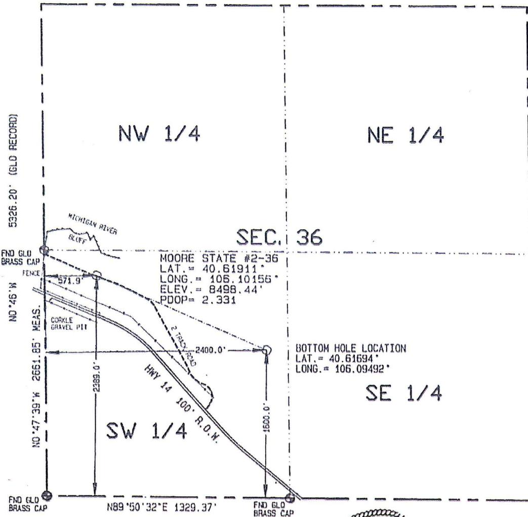
BASIS OF BEARINGS IS THE WEST LINE OF THE SW 1/4 OF SEC. 36, T8N, R78W OF THE 6TH P.M. JACKSON COUNTY, CO. BEARS N00°47'39"E BETWEEN SET MONUMENTS AS DETERMINED BY GPS (NAD 83)
