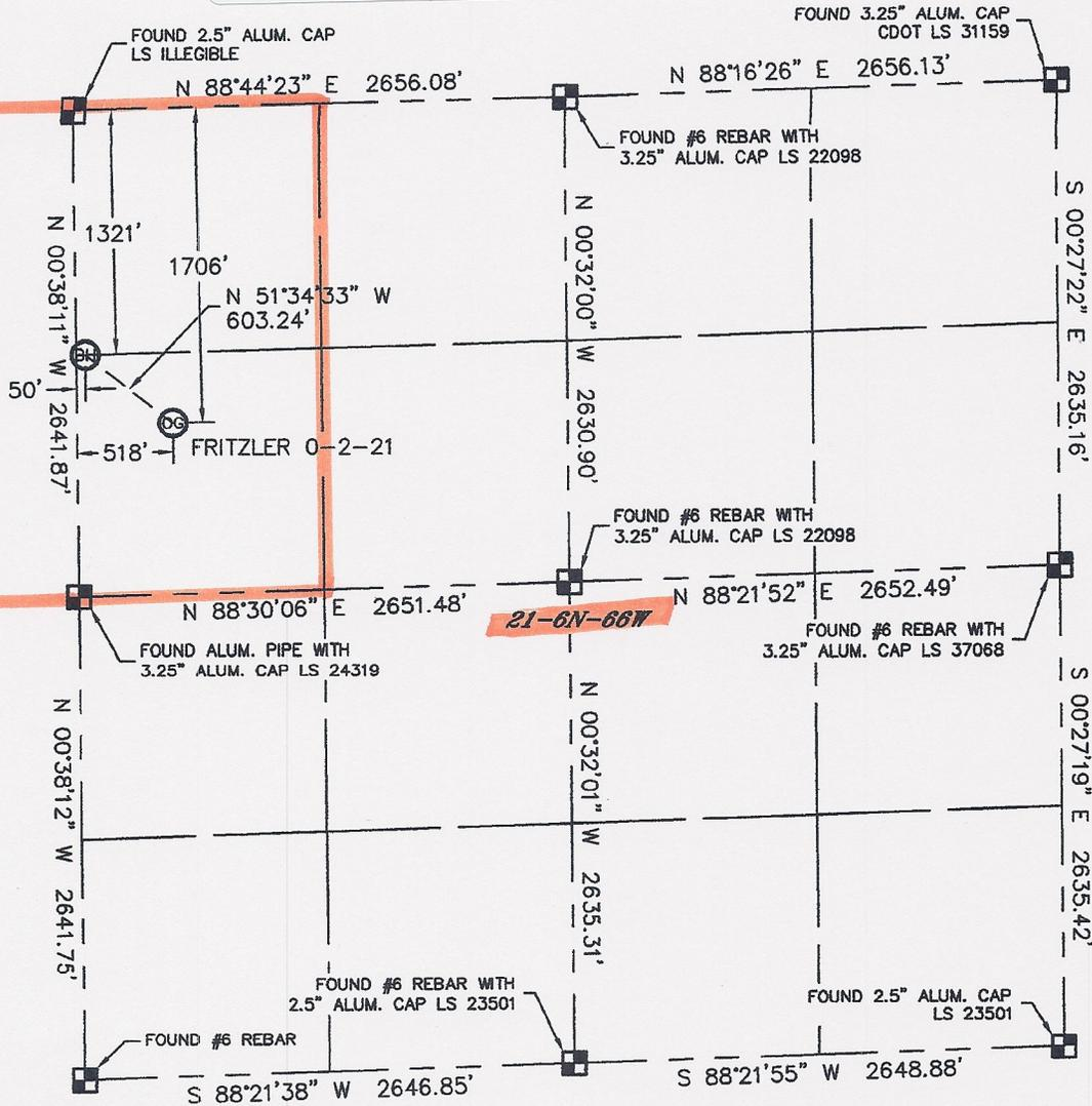
In accordance with a request from ANDY PETERSON with HRM RESOURCES, LLC Lat40°, LLC has determined the surface location of the FRITZLER 0-2-21 to be 1706' from the NORTH line and 518' from the WEST line and the bottom hole to be 1321' from the NORTH line and 50' from the WEST line as measured at right angles from the section lines of Section 21, Township 6 North, Range 66 West of the Sixth Principal Meridian, County of Weld, State of Colorado.
