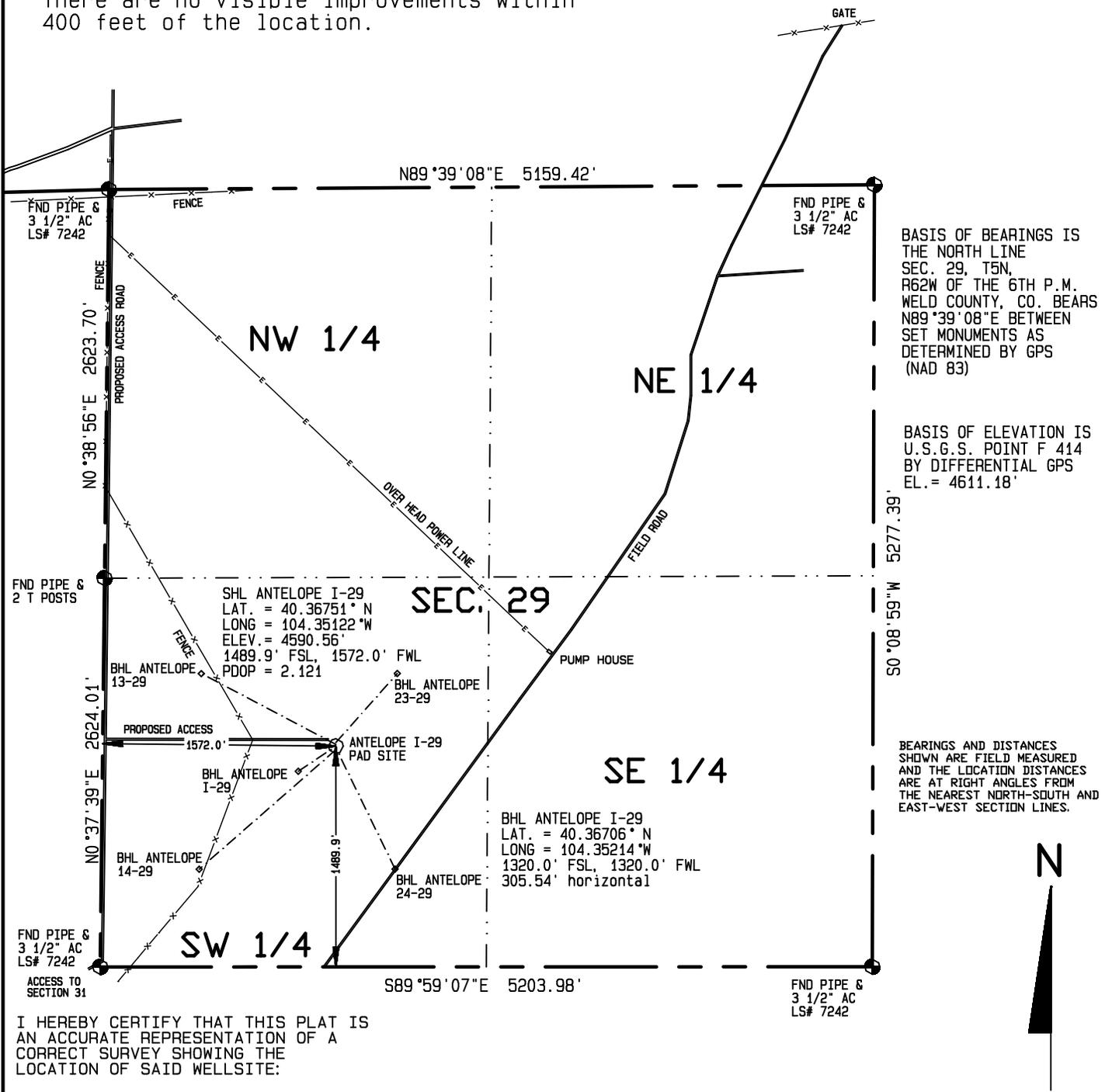
BASIS OF BEARINGS IS THE NORTH LINE SEC. 29, T5N, R62W OF THE 6TH P.M. WELD COUNTY, CO. BEARS N89°39'08"E BETWEEN SET MONUMENTS AS DETERMINED BY GPS (NAD 83)
