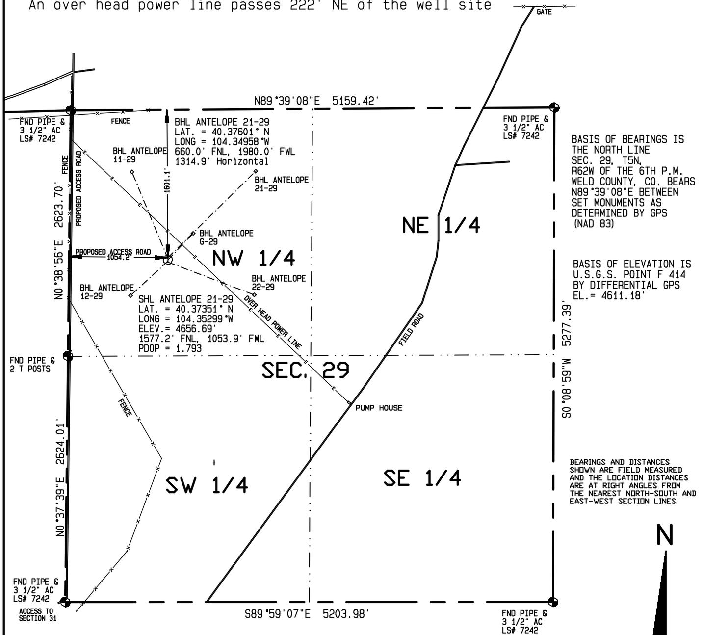
BASIS OF BEARINGS IS THE NORTH LINE SEC. 29, T5N, R62W OF THE 6TH P.M. WELD COUNTY, CO. BEARS N89°39'08"E BETWEEN SET MONUMENTS AS DETERMINED BY GPS (NAD 83)
