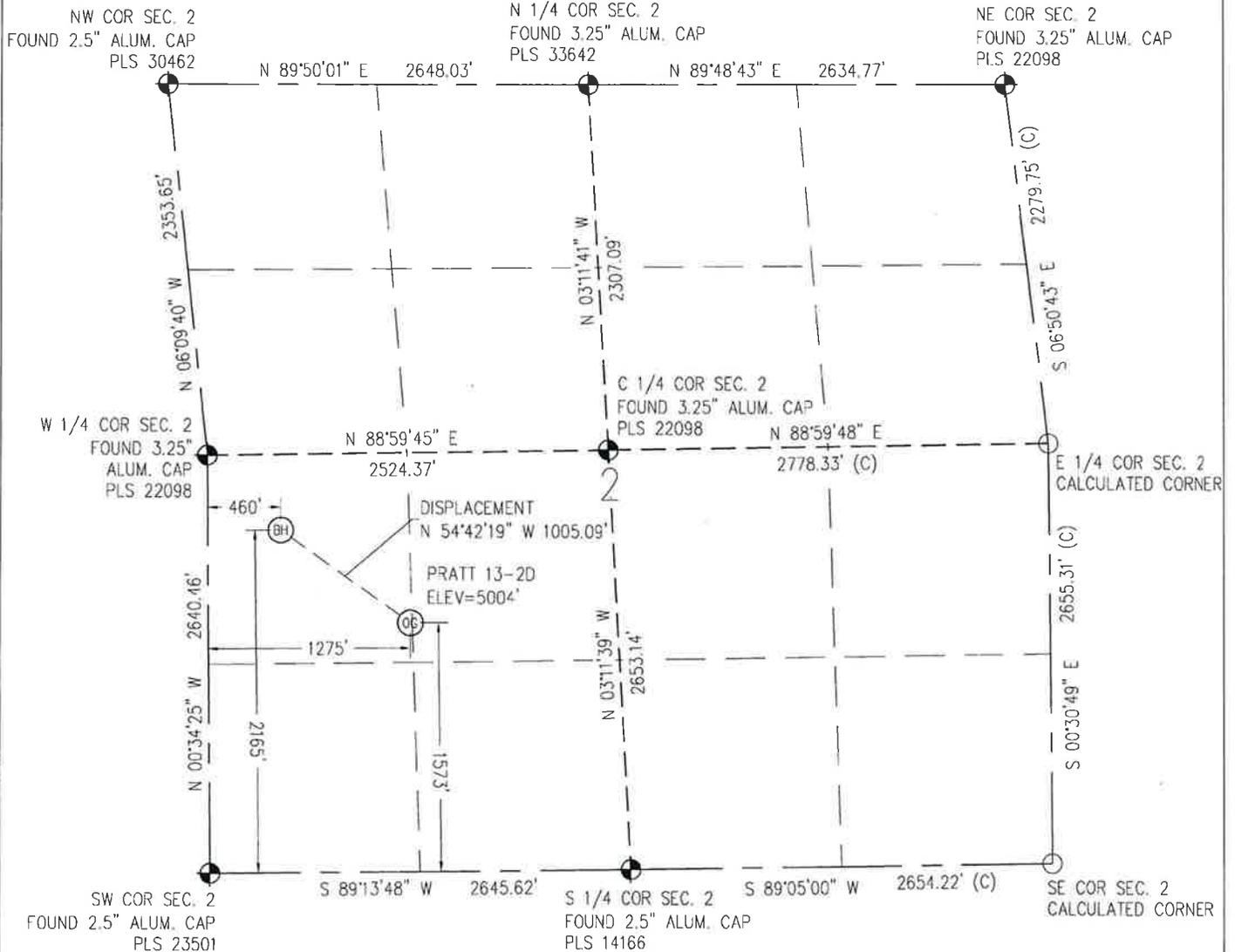
IN ACCORDANCE WITH A REQUEST FROM CRAIG RASMUSON - SYNERGY RESOURCES, BASELINE ENGINEERING CORP. HAS DETERMINED THE LOCATION OF THE PRATT 13-2D TO BE 1573' FSL AND 1275' FWL, AS MEASURED AT NINETY (90) DEGREES FROM THE SECTION LINE OF SECTION 2, TOWNSHIP 4 NORTH, RANGE 68 WEST AND THE BOTTOM HOLE LOCATION TO BE 2165' FSL AND 460' FWL OF SECTION 2, TOWNSHIP 4 NORTH, RANGE 68 WEST, 6TH PRINCIPAL MERIDIAN, WELD COUNTY, COLORADO.
