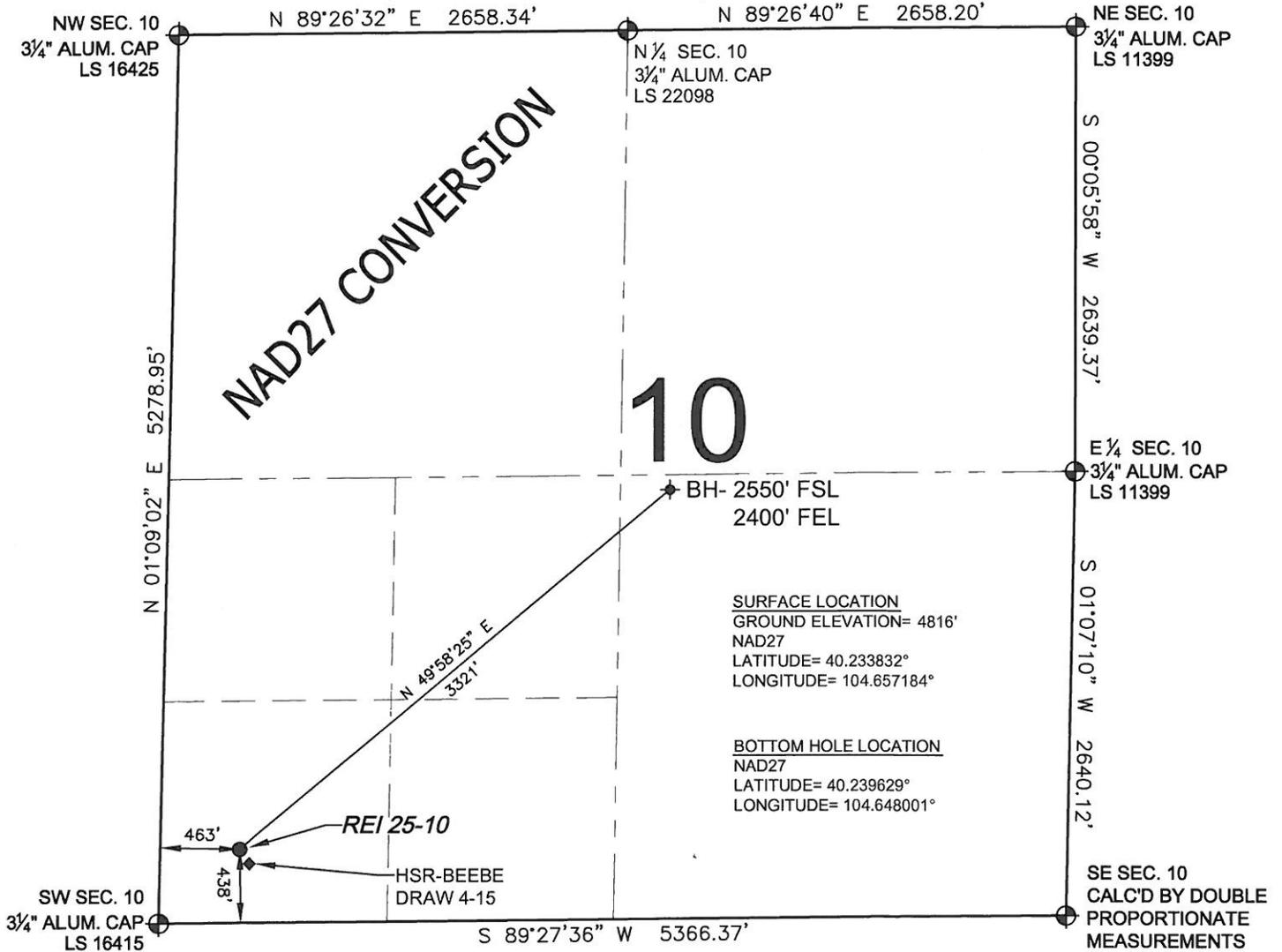
**WELL REI 25-10 TO BE LOCATED 438' FSL AND 463' FWL, SECTION 10, T3N, R65W OF THE 6th P.M.**
