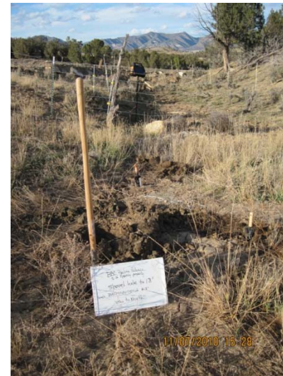
COGCC-2 Soil Sampling Location @ 18" below ground level (shovel in hole)
