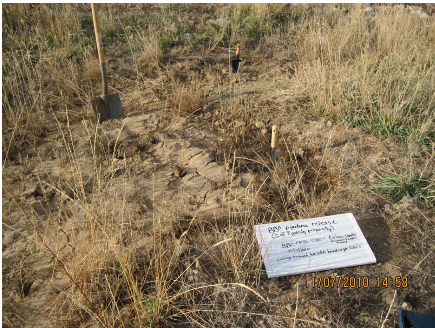
Proximity of sample locations: Wood Handled Trowel At COGCC1 sample location (surface sample), Shovel At COGCC2 sample location (18" depth), Orange Handled Trowel At HAW sample location (water in hole ~1 ft deep)
