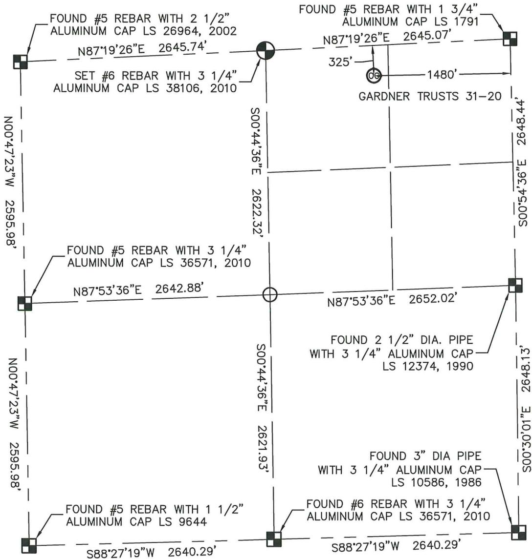
In accordance with a request from DAVID LEDET with NOBLE ENERGY INC. King Surveyors Inc. has determined the surface location of GARDNER TRUSTS 31-20 to be 325' from the NORTH line and 1480' from the EAST line, as measured at right angle, from the section lines of Section 20, Township 2 North, Range 46 West of the Sixth Principal Meridian, County of Yuma, State of Colorado.
