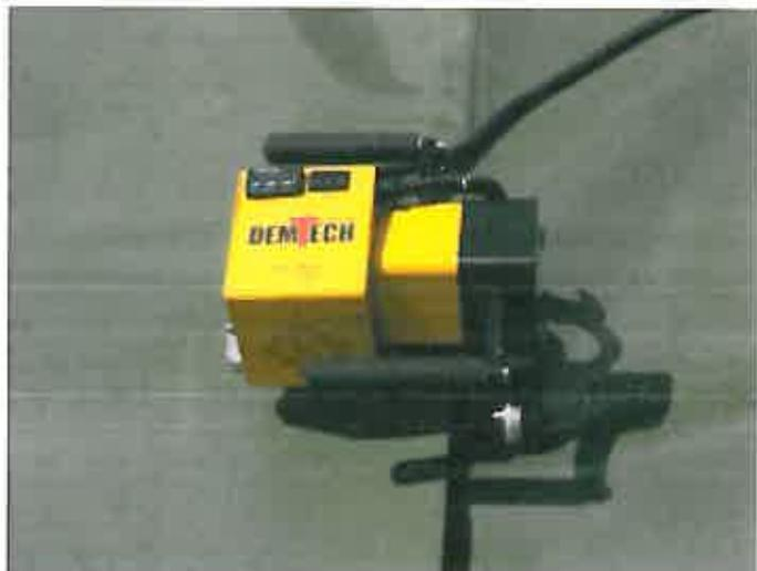
(B) Extrusion fillet welding consists of extruding a bead of molten resin along the edge of a panel lapped on top of another panel. The molten resin causes the melting of each sheet, which results in a homogeneous bonding of the panels. The polyethylene rod used for welding must be compatible with the liner material.
