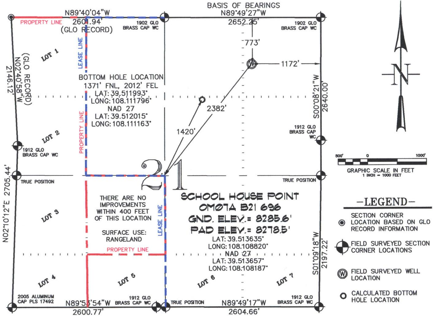
**THIS WELL LOCATION PLAT WAS PREPARED FOR BERRY PETROLEUM COMPANY TO LOCATE THE SCHOOL HOUSE POINT OM07A B21 696 WELL, 773 FEET FROM THE NORTH LINE AND 1172 FEET FROM THE EAST LINE IN THE NE1/4 NE1/4 OF SECTION 21, T. 6 S., R. 96 W. OF THE 6TH P.M. GARFIELD COUNTY, COLORADO.**
