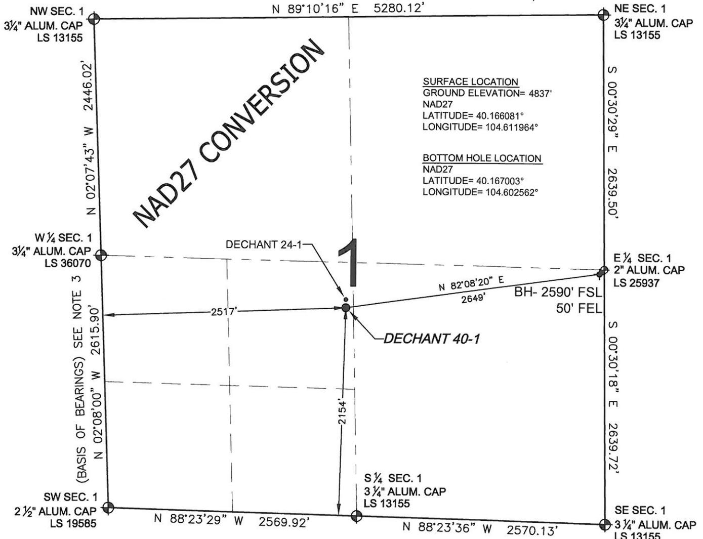
**WELL DECHANT 40-1 TO BE LOCATED 2154' FSL AND 2517' FWL, SECTION 1, T2N, R65W OF THE 6TH P.M.**
