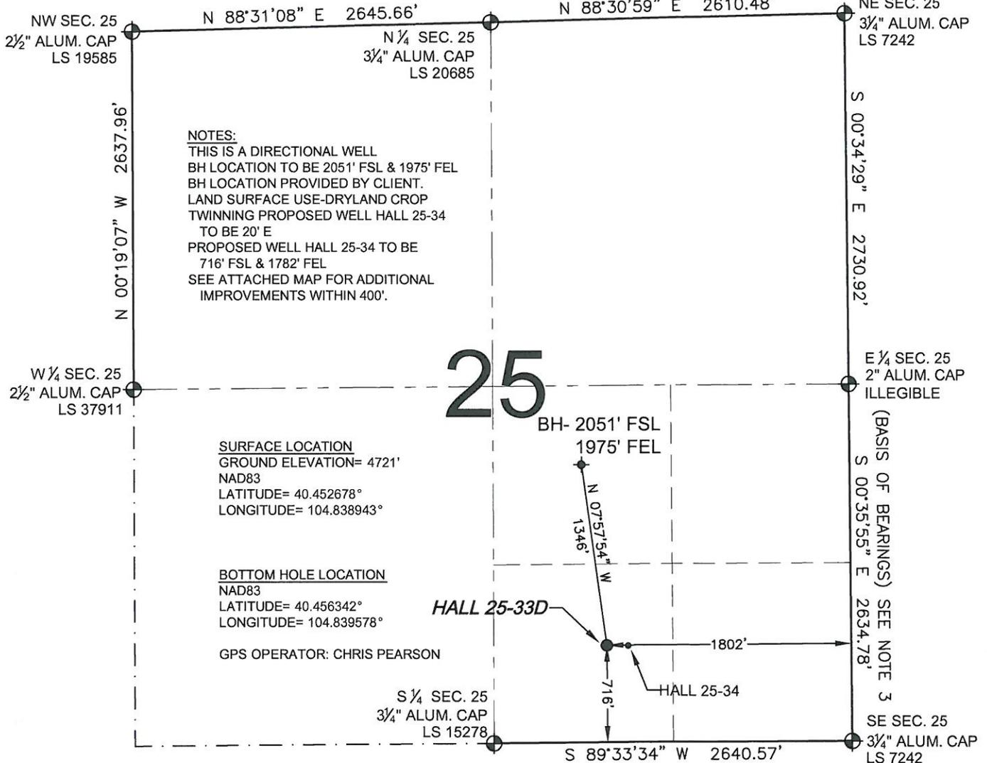
WELL HALL 25-33D TO BE LOCATED 716' FSL AND 1802' FEL, SECTION 25, T6N, R67W OF THE 6th P.M.
