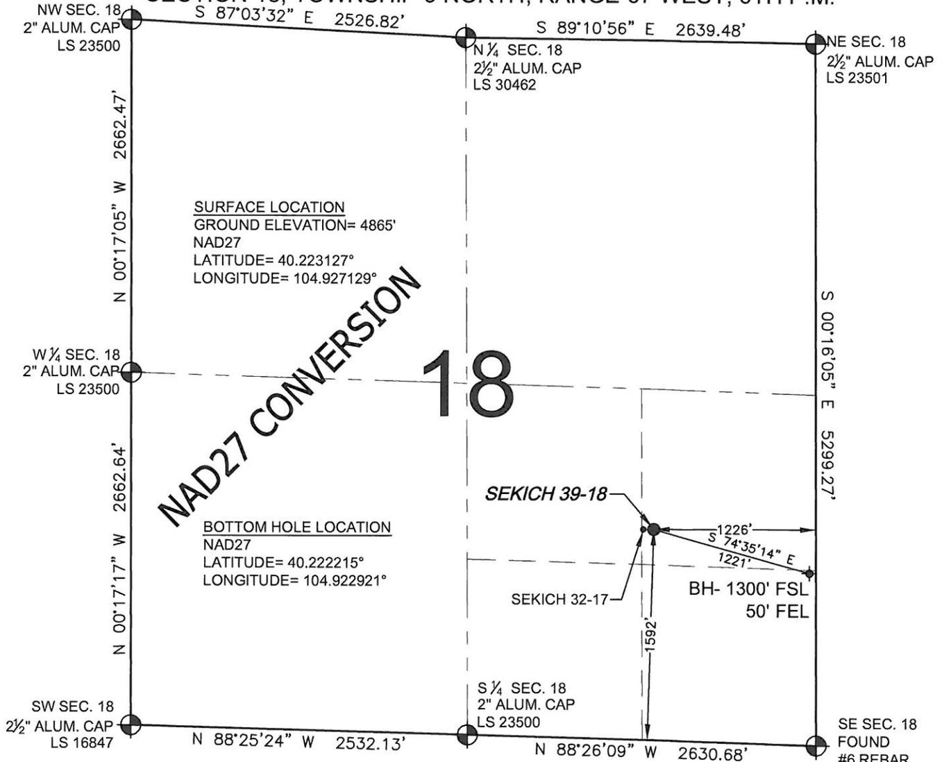
WELL SEKICH 39-18 TO BE LOCATED 1592' FSL AND 1226' FEL, SECTION 18, T3N, R67W OF THE 6th P.M.
