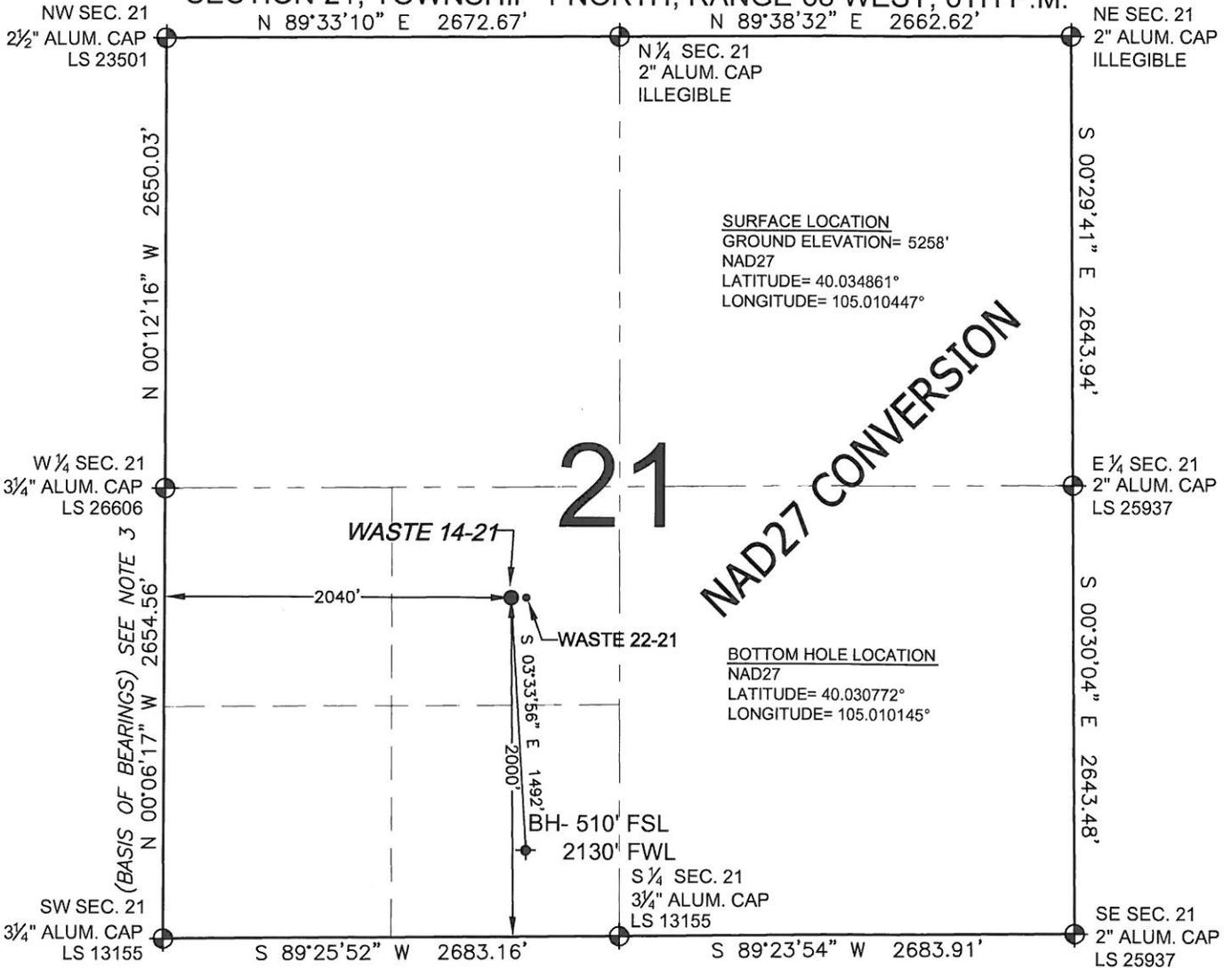
WELL WASTE 14-21 TO BE LOCATED 2000' FSL AND 2040' FWL, SECTION 21, T1N, R68W OF THE 6th P.M.
