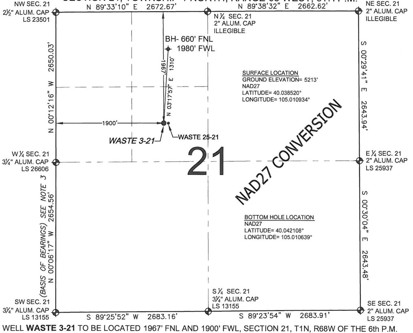
WELL WASTE 3-21 TO BE LOCATED 1967' FNL AND 1900' FWL, SECTION 21, T1N, R68W OF THE 6th P.M.
