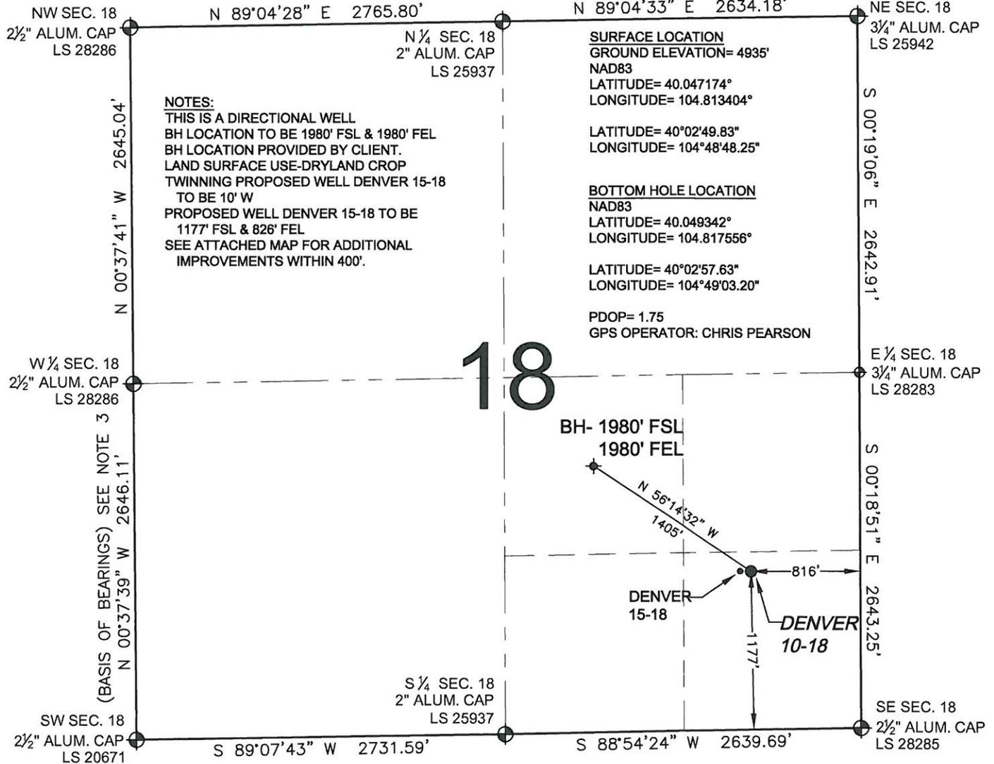
WELL DENVER 10-18 TO BE LOCATED 1177' FSL AND 816' FEL, SECTION 18, T1N, R66W OF THE 6th P.M.
