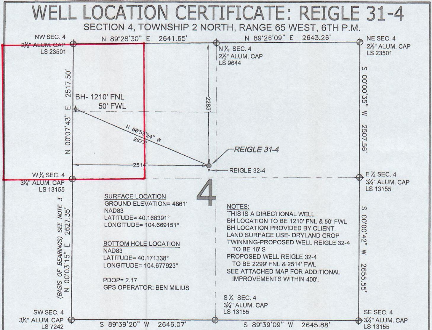
WELL REIGLE 31-4 TO BE LOCATED 2283' FNL AND 2514' FWL, SECTION 4, T2N, R65W OF THE 6th P.M.
