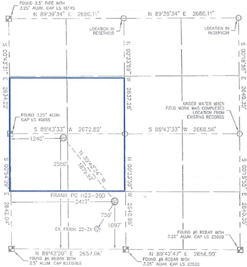
In accordance with a request from JOE JOHNSON with Noble Energy Inc., Lat40°, LLC has determined the surface location of the FRANK PG H22-20D to be 1097' from the SOUTH line and 2417' from the WEST line and the bottom hole to be 2550' from the SOUTH line and 1240' from the WEST line as measured at right angles from the section lines of Section 22, Township 3 North, Range 65 West of the Sixth Principal Meridian, County of Weld, State of Colorado.
