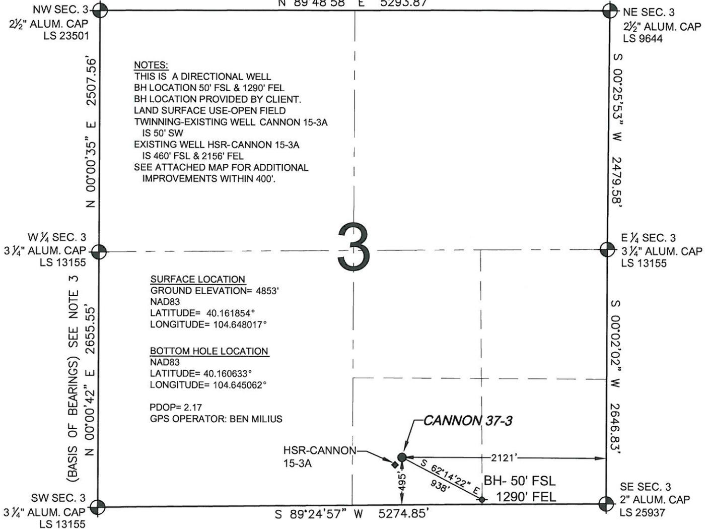
WELL **CANNON 37-3** TO BE LOCATED 495' FSL AND 2121' FEL, SECTION 3, T2N, R65W OF THE 6th P.M.
