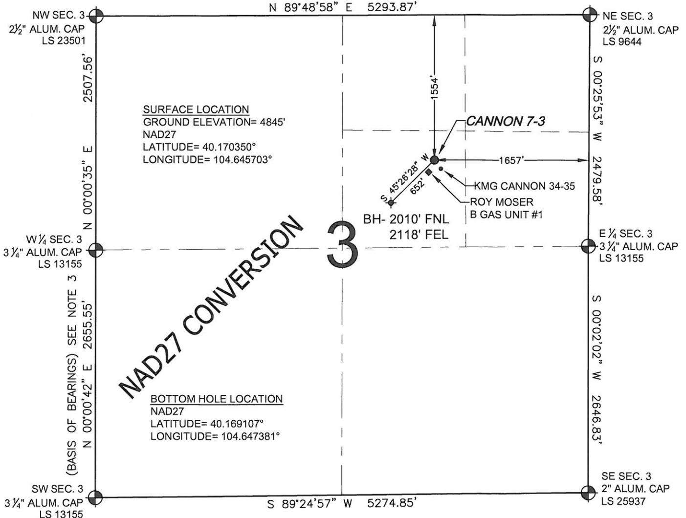
WELL **CANNON 7-3** TO BE LOCATED 1554' FNL AND 1657' FEL, SECTION 3, T2N, R65W OF THE 6th P.M.
