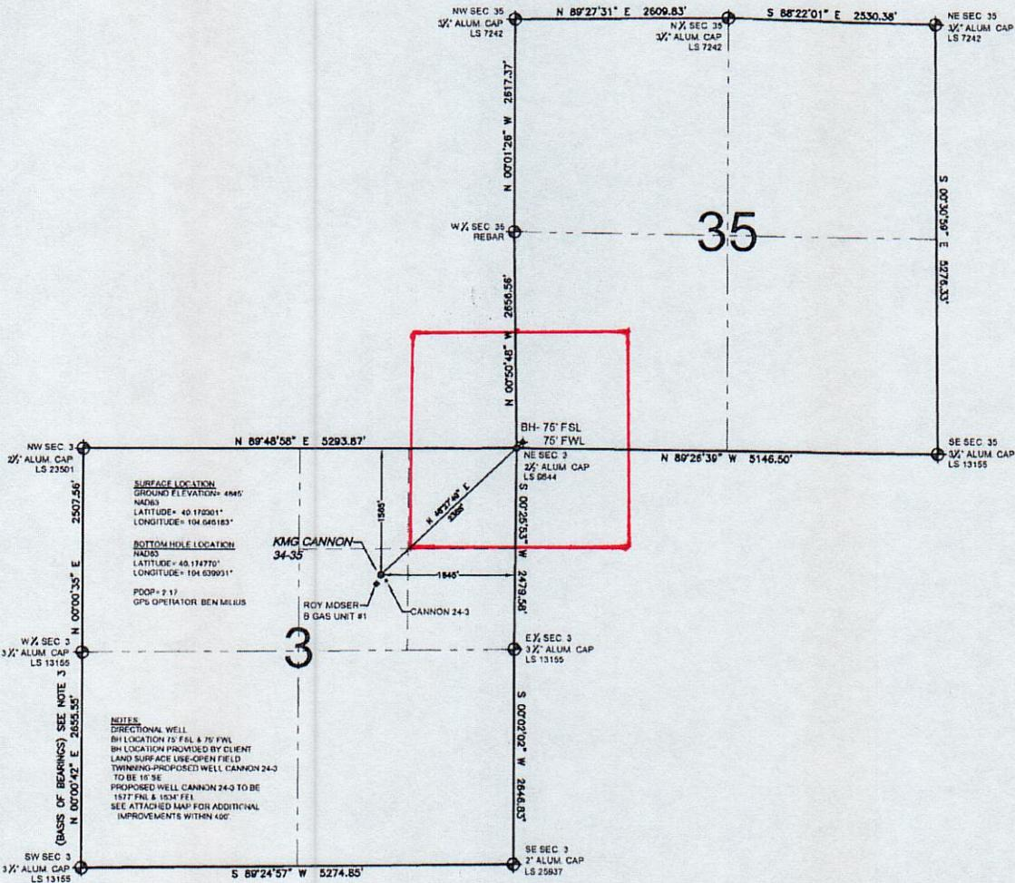
WELL KMG CANNON 34-35 TO BE LOCATED 1565' FNL AND 1645' FEL, SECTION 3, T2N, R65W OF THE 6th P.M.
