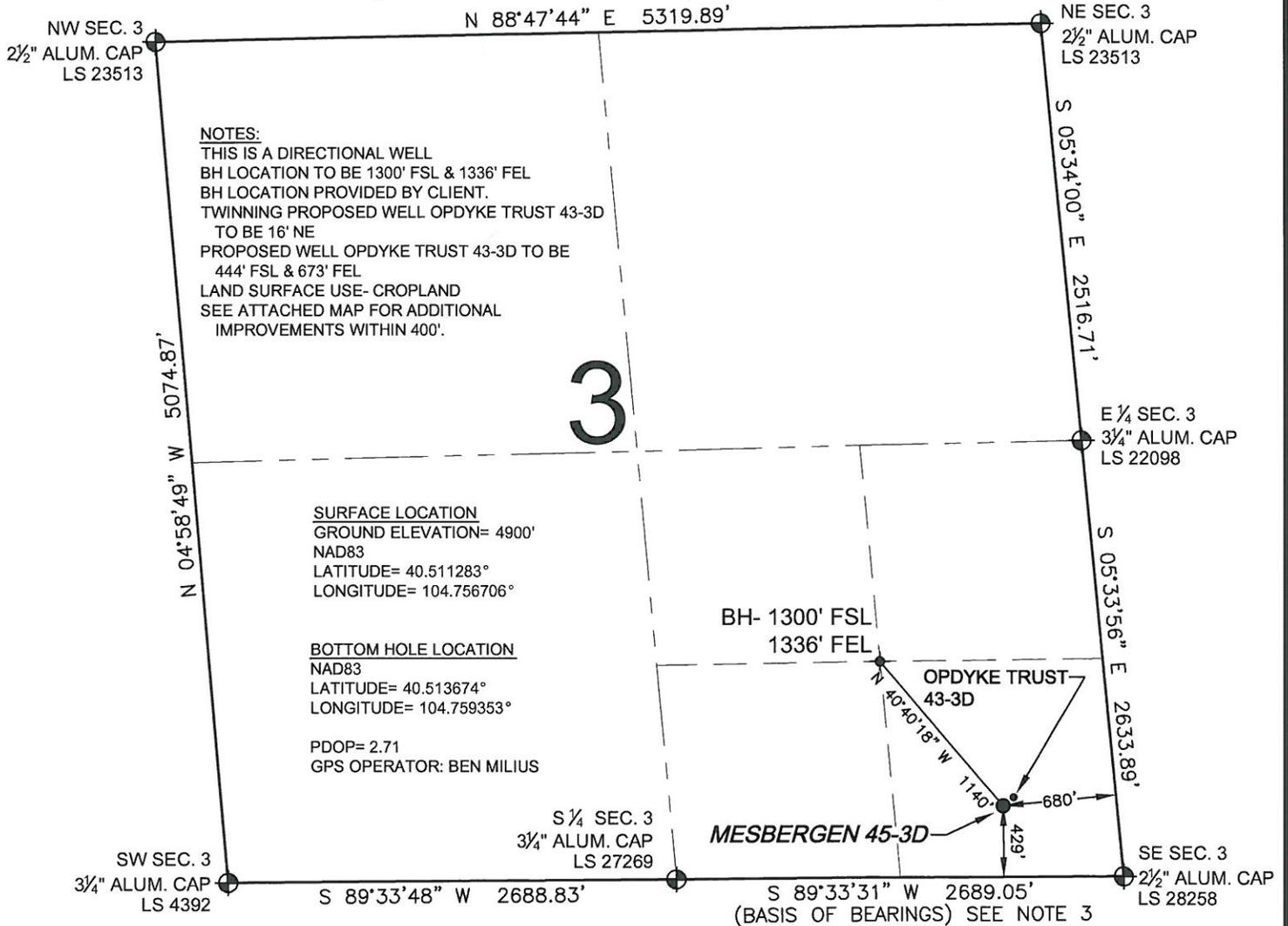
WELL **MESBERGEN 45-3D** TO BE LOCATED 429' FSL AND 680' FEL, SECTION 3, T6N, R66W OF THE 6th P.M.
