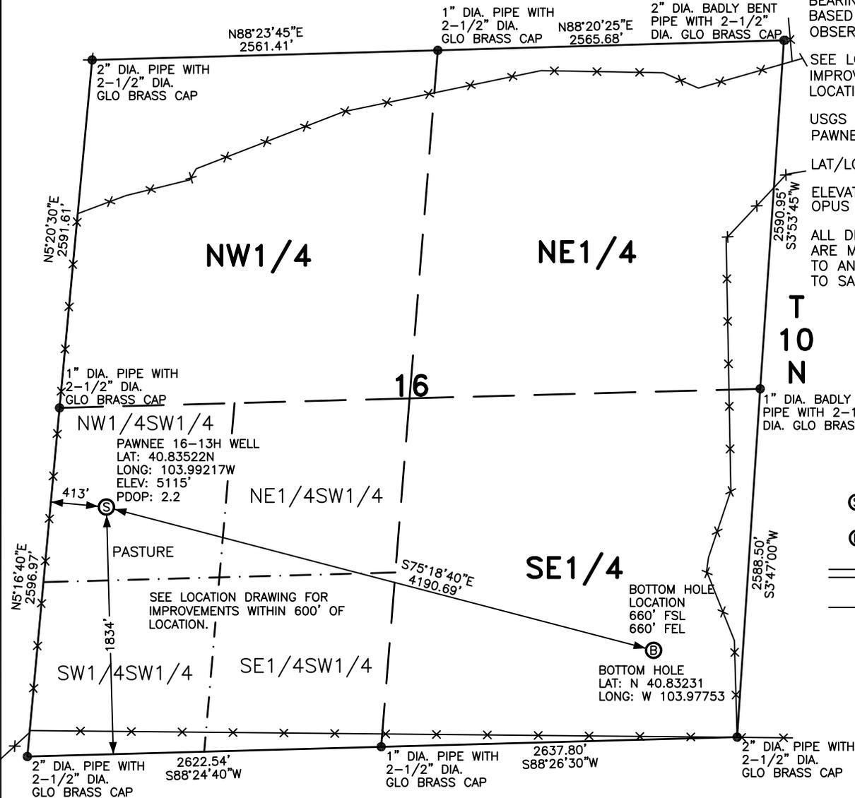
THIS WELL LOCATION PLAT HAS BEEN PREPARED FOR WHITING OIL AND GAS CORPORATION, TO LOCATE THE PAWNEE 16-13H WELL BEING 413 FEET FROM THE WEST LINE AND 1834 FEET FROM THE SOUTH LINE IN THE NW1/4SW1/4 OF SECTION 16, TOWNSHIP 10 NORTH, RANGE 59 WEST OF THE 6TH P.M., WELD COUNTY, COLORADO. THE SURFACE ELEVATION AT THIS POINT IS 5115 FEET. THIS IS NOT A LAND SURVEY PLAT.
